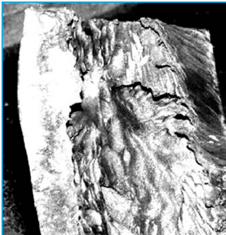
Photo 2. Erosion of Standard API 610 Pump
